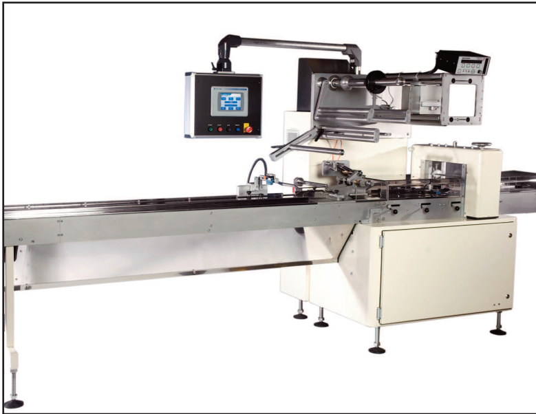
GSD wrote the software for the servo controller and HMI (human-machine interface) for this flow wrapping machine by Daco Packaging.
